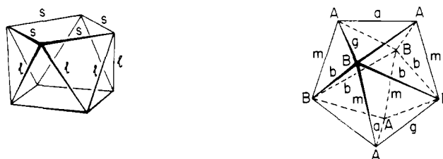
Figure 4. The D_{4d} square antiprism and the D_{2d} dodecahedron with vertices and edges labeled according to Hoard and Silverton. 26
